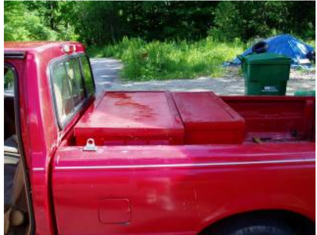
The Ford Ranger has limited space under the bed – these batteries are in the bed.
