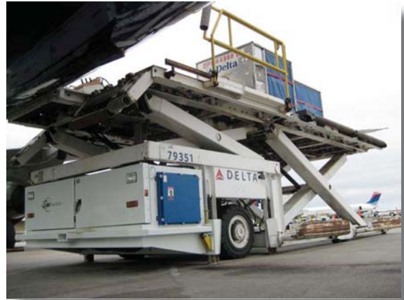
1996 C15 cargo loader converted from diesel to electric, in operation at Atlanta-Hartsfield International Airport
